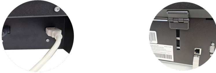
Shows the locations of the USB port connectors on the embosser and ink attachment
