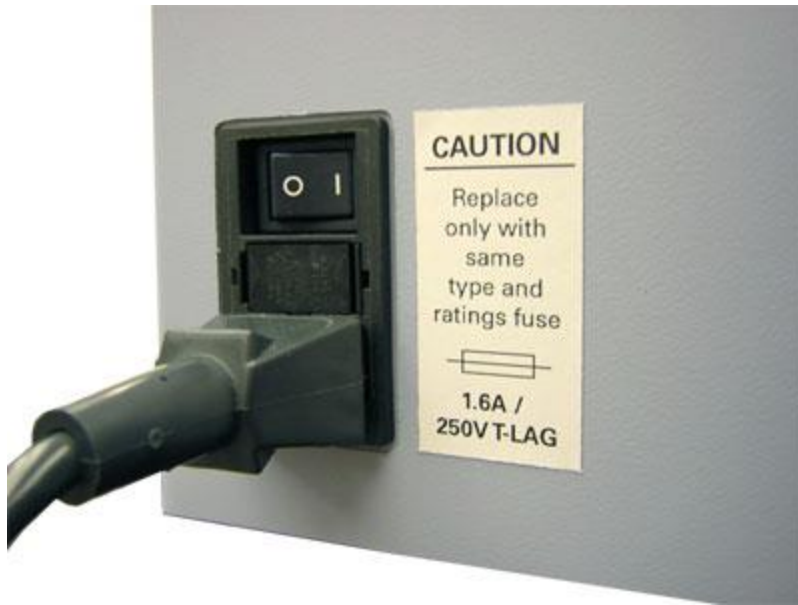
Shows the power switch in the back of the embossing printer
