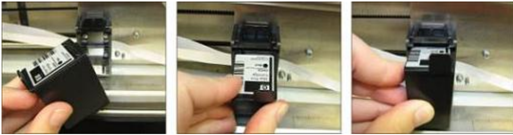
Shows how to insert an ink cartridge
