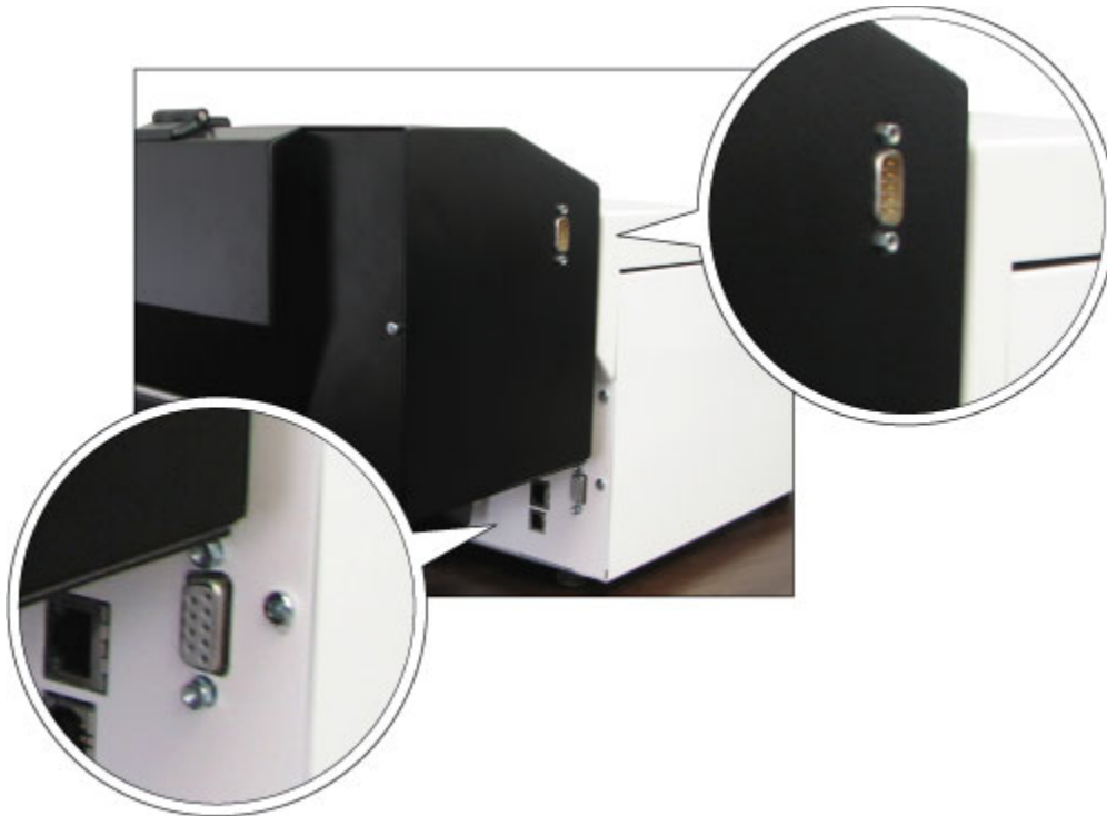
Shows the locations of the serial port connectors on the embosser and ink attachment
