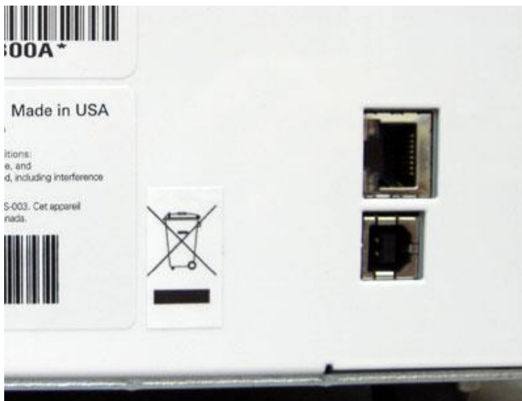
Shows the USB and LAN connectors in the back of the embosser
